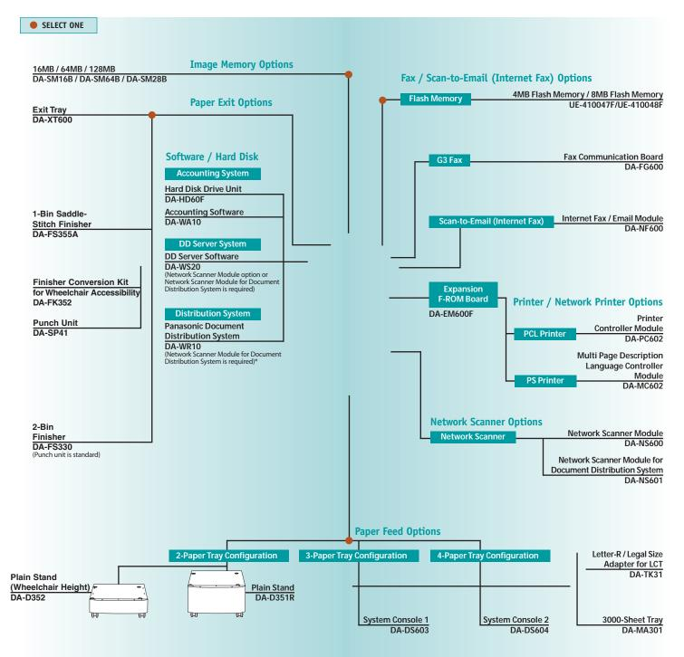
\*If the distribution of G3 Fax data is necessary, Fax Communication Board (DA-FG600) and Internet Fax / Email Module (DA-NF600) are required. \*If the distribution of Internet Fax data is necessary, Internet Fax / Email Module (DA-NF600) is required.
